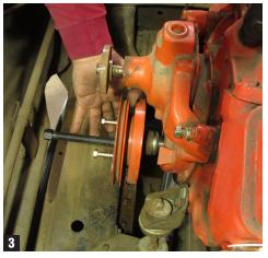
3. CPP's #18-35 harmonic balancer (6-1/8" diameter, 3/4" thick) replaces the early integrated balancer; it's slightly more offset, which benefits pulley spacing, however the timing mark matches up identically. (Fig 4)
