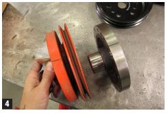
4. The existing pilot hole will initially determine how the job proceedsif it's not deep enough, getting your drill's pilot hole dead-center may be difficult (without having to machine an addition guide to drill a
