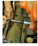
11. After cutting the initial half-inch of threads, remove sleeve/bushing and finish remaining depth. (Fig. 14)
