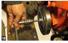
If you've already removed the stock balancer, you will need to use a sleeve guide (steel tubing) to stabilize bushing during drilling/tapping. That translated into a piece of 1/8-inch-wall 1-1/2-inch tube, slotted for the crankshaft keyway. (Fig. 11)
