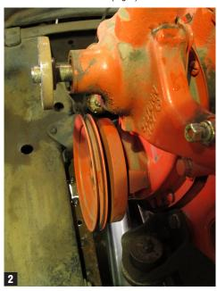
2. Removal of the early-style dampers/pulleys is no different than removing a later-style balancer (using a puller); it's the reinstallation that ultimately necessitates the drilling/tapping of the crank snout. (Fig 3)
