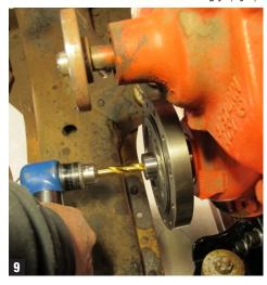
Start tapping the threads (using the tap bushing) once the hole has been drilled to depth; keep tap well lubricated with cutting fluid and periodically clean off debris. Cut approximately a half-inch deep, just enough to stabilize tap without bushing. (Fig. 10)
