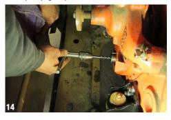
12. Always keep the tap welloiled with cutting fluid and wipe off the metal debris regularly to ensure your crank threads are sharp and clean. Install the new balancer bolt prior to putting the balancer on to verify threads are accurate. (Fig. 15)
