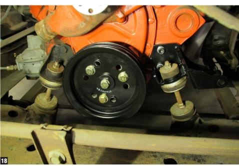
15. Install new pulley(s) and secure with new balancer bolt, spacer, and lock washer. (Fig 18)
