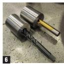
6. The bushings are machined to fit the ID of the balancer mounting hole (1.225"). The inner lip of the balancer may require slight cleaning up with a file or sand paper if it's been hammered on in the past. (Figs. 7-8)
