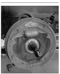
The passenger-side brake didn't look all that bad, except for the fact that the secondary shoes were used both front and rear (the primary or forward shoe should have the shorter lining
