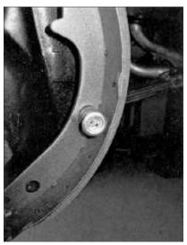
... they get replaced with the modernstyle coil-spring retainers LMC supplies with its rebuild components.
