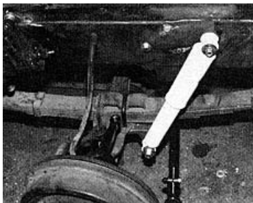
This is how the shock will look when installed properly.
