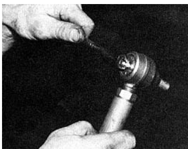
Install the provided Zerk fittings into the rod ends of the drag link.
