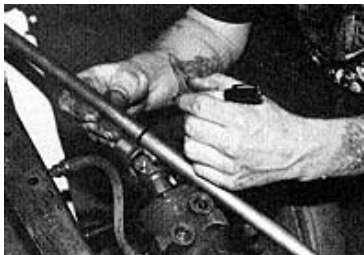
This is what the steering box will look like installed with the steering shaft attached.
