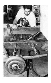
Now you can slide the complete power steering setup under the truck, behind the axle.
