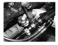
The new control valve simply installs right onto the stock pitman arm in the same fashion as the tie rod ends and drag link.
