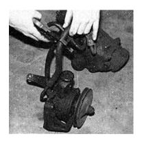
The choice of power steering pump will be determined by what engine your truck has. In this case, we are using a pump for a small block Chevy which is common with customizers. A quick trip to the parts yard will surely yield the pump you need. It is important that you get the hoses with the pump to continue the installation.
