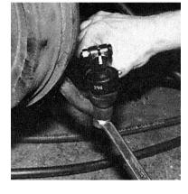
Install each new OEM upgrade one-inch tie rod ends onto the top of the steering arms that you removed the ball ends from. Cotter pins are to be installed here too.
