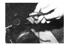
Cut the pressure hose to the required length and screw on the threaded nut (left hand threads).
