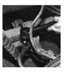
The new drag link extending from the control valve is then installed onto the steering arm in the same manner as the stock drag link. Once again, be sure to install the cotter pins.
