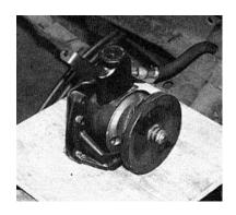
Since this truck doesn't have an engine, we are going to dummy where the pump will probably be mounted so that the hoses will be of proper length.
