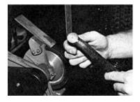
Using the belt sander, remove the pressed edge to the point where you can slightly notice the outer circumference of the ball joint.
