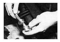
The re-usable fitting and nipple are then installed into the nut.
