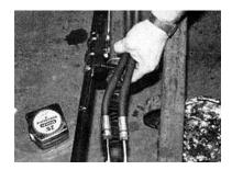
Using a grease gun, lube all zerk fittings on the assembly (as well as your stock fittings while you're at it) to obtain the most from this system.
