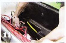
11. Place the gearbox into the car and align the bolt holes. You will most likely find that your wheel housing must be trimmed for clearance of the new gearbox. If so, mark and trim the wheel housing to fit. Once it fits, bolt your new gearbox into place.
