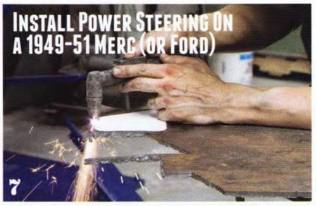
7. Transfer the template to the 1/4" plate and cut. Then drill out all holes to 3/8". You'll want to countersink the two holes going into the new gear box so that the 3/8" flathead socket cap screws will mount flush.
