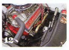
12. Connect the new Vega Pitman arm, then mount the new power steering pump brackets and pump. Attach the hydraulic lines and fill the pump, check for leaks.
