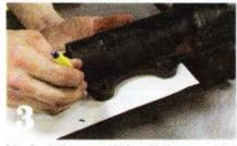
ble check that your holes all line up with your gearboxes, repeat this process to make a template for the new gearbox. Cut out the outline of both templates, then align them using the bolt holes and trace the outline onto the poster board.
