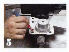
5. Place the final template onto the new gearbox and align all of the holes. You will notice one hole is blocked. Mark that blocked hole with a paint marker.
