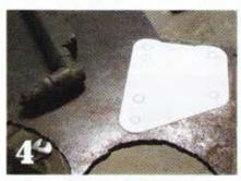
4. Cut the finished template (here the template is laid on the 1" steel we'll make the bracket from). Place your template on the frame side and slip the 3 bolts through the holes. (You may find that the template interferes with the pressure
