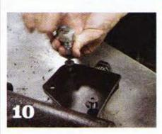
Mount the adapter plate to the new power steering gearbox.
