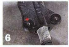
6. Remove the template and grind a flat spot to drill where the paint mark is. Replace the template and use a punch to mark the center of the hole. Drill and tap the hole out to 3/8-16 thread.
