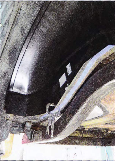
8. The new wheel housing was mocked in place ...
