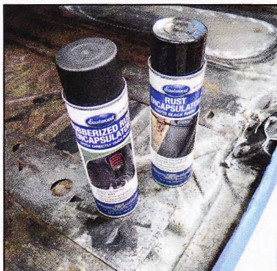
27. Eastwood Rust Encapsulator was used; the regular product used inside, and the rubberized version used on the underside, as it acts as an undercoating.
