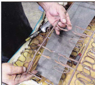
27. Eastwood Rust Encapsulator was used; the regular product used inside, and the rubberized version used on the underside, as it acts as an undercoating.
