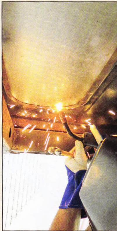
The edge was also welded on the underside in sections.
