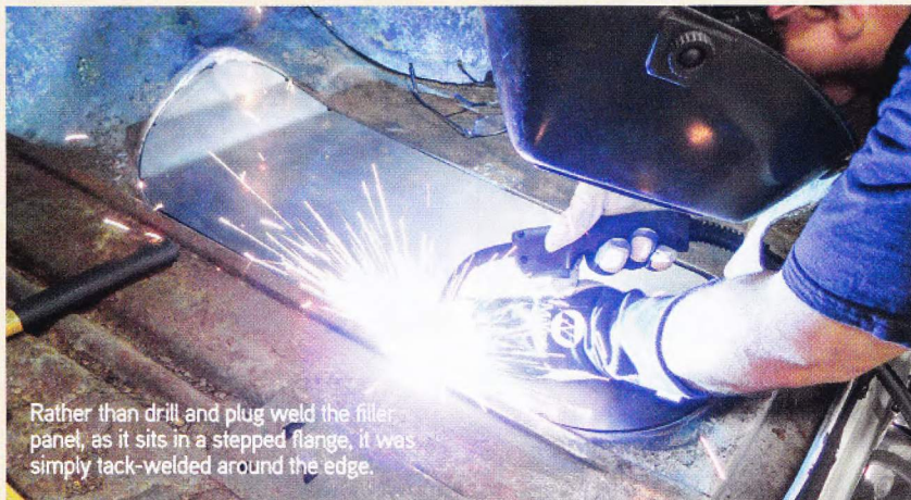
This simple, 18-gauge filler panel was cut to size and bent to shape at its forward edge, then checked for fit one final time.
