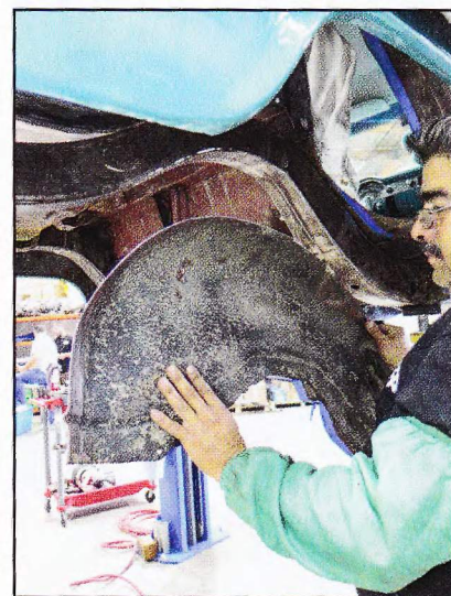
15. The original inner wheelwell was then removed in one piece.
