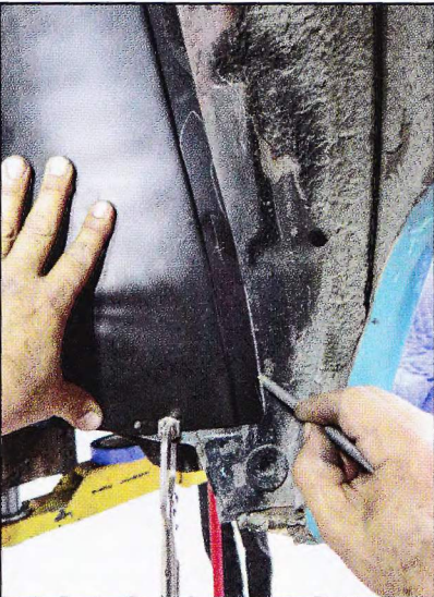
9. ... and the outer profile, toward the fender lip, was transferred onto the original wheelwell.
