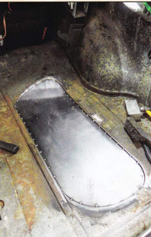
The panel tack-welded in place. It was further welded in short sections between the tacks.
