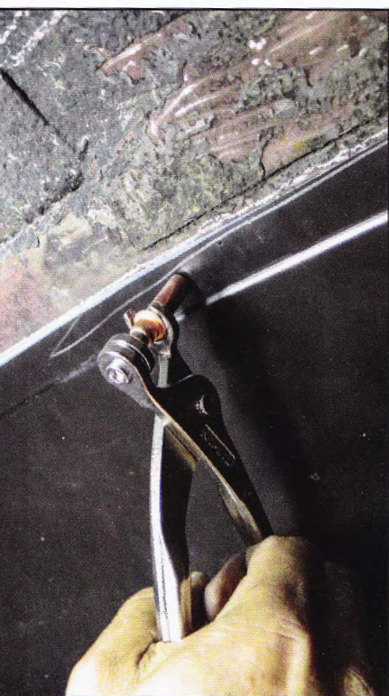
19. Once happy with the fit of the new panel, it was temporarily attached through the overlap using Cleco fasteners.
