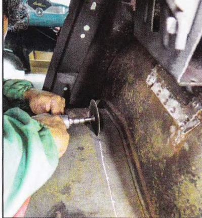
13. The same process was repeated on a line marked between the previously drilled holes on the trunk floor.
