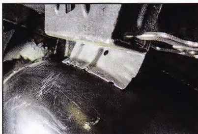
24. The trunk hinge brace, shown cut at the old spot-weld points, was recontoured to fit the shape of the new panel before being welded in place.
