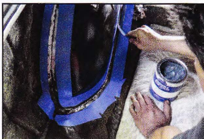
25. Once the panel was finish welded all round and the Cleco holes welded shut, Eastwood seam sealer was applied over the joints. The masking tape makes for neat edges to the sealer once it is brushed on.
