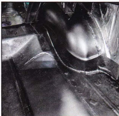
28. The Rust Encapsulator was applied to the wheelwells, floor, and inner quarter-panels.
