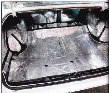
29. Hushmat was then installed on all trunk surfaces, as well as the underside of the trunklid itself.
