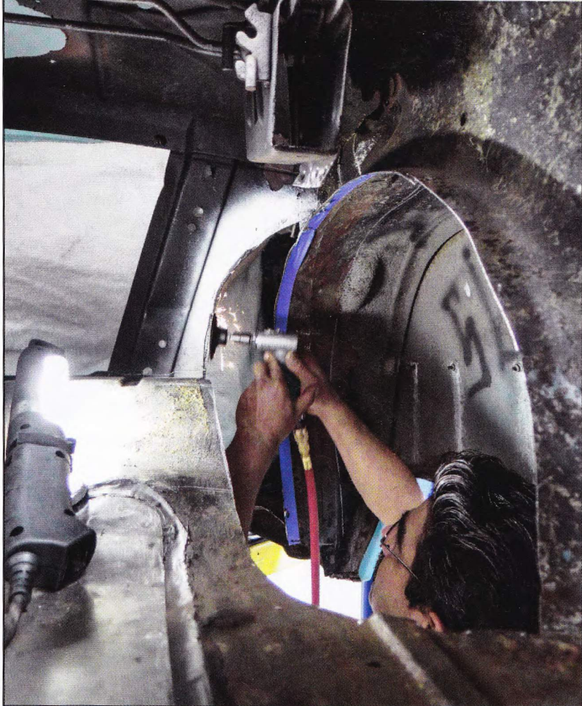
18. ... then dressed with a small air grinder.
