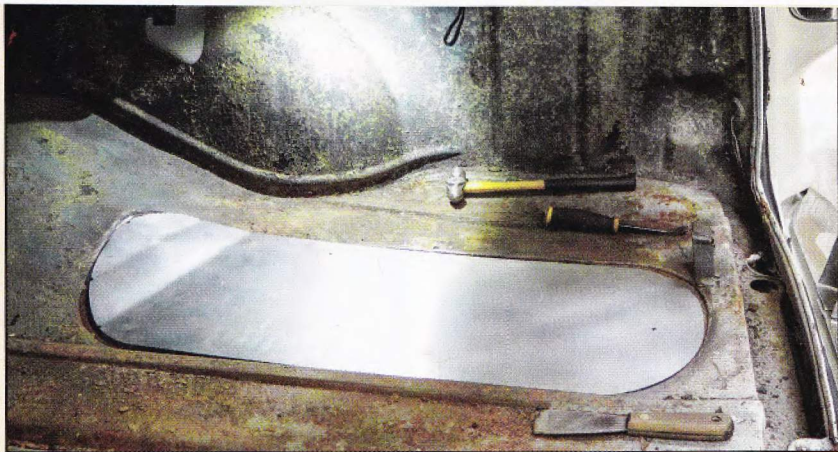
This simple, 18-gauge filler panel was cut to size and bent to shape at its forward edge, then checked for fit one final time.
