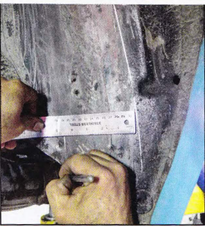
10. From there, a "rough" cut line was established, factoring in the added width of the new wheel housing minus the overlap.
