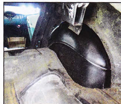
16. Since the opening was cut undersize, the wider wheel housing was mocked in place to determine further trimming.
