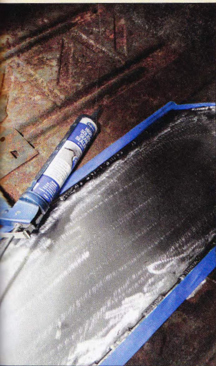
Eastwood high solid seam sealer was used to seal the perimeter. Note the short sections of weld rather than just tacks. The sealer will prevent moisture and rust in the joint.
