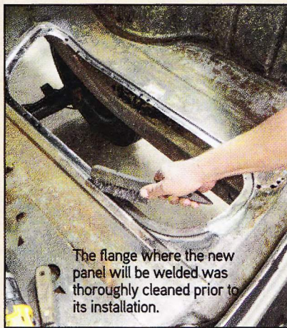
Once all the spot welds were drilled out, the wheelwell was removed.
