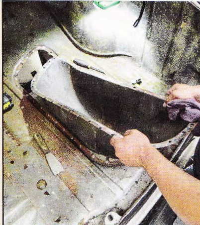
Once all the spot welds were drilled out, the wheelwell was removed.
