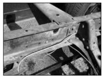
We started with a '56 F-100 frame that was missing the stock, single-brake master cylinder, with a clutch and brake-pedal assembly. Note the 1-inch hole provided for the stock clutch pedal.
