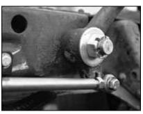
The CPP pushrod was attached to the lower hole in the stock Ford brake pedal using special Grade 8 hardware included in CPP's kit.
