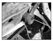
We removed the shaft, and left the Ford stock brake pedal mounted on the stock master cylinder mount.
