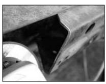
A test fit of the CPP bracket revealed that years of use had changed (bent) some of the original dimensions of the Ford chassis. Using a body grinder, we ground off the front of the Ford bracket.
