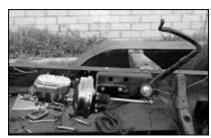
Paying close attention to how well existing Ford holes, and the CPP mounting bracket, lined up paid off with a real clean installation. Now that we have the right dual master cylinder and power-brake booster in place, we can move on to the right setup for the rear discs.
