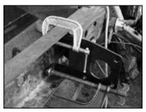
Before drilling the two 3/8-inch holes required to mount the CPP bracket to the frame, we used C-clamps and the CPP bracket as a drill template.
