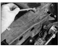
To ensure that the CPP mounting bracket would properly line up, we first double-checked to see that the stock Ford bracket was tightly bolted
