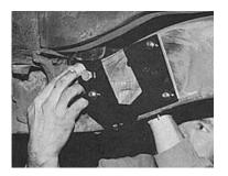
When you have the new holes drilled, reverse the bolts so that they are inserted from the inside of the frame. Three of the bolts extend outward as shown. The upper left hand bolt is still a bracket locater bolt so it remains installed from the outside. Also, take note of the lower hole that meets at the bottom of the frame. This hole is threaded because there is no frame to drill through.
