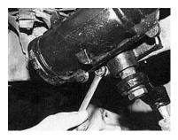
While someone tightens the inner bolts into the gearbox, notice that the lower hole that you drilled out secures a bolt that is installed from the outside of the frame into the threaded bracket.
