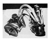
You must come up with the 1969-'87 2wd half-ton Chevy truck power steering box and pitman arm, matching hose kit and power steering pump. Take note of exactly what year box you have so that you can get the same year hose kit and power steering pump from your local parts supplier. In
