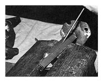
Classic Performance Products even includes a one-half-inch section of angle iron that is used to help you scribe an alignment mark on the steering shaft.
