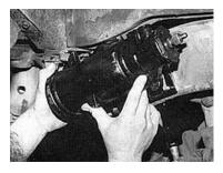
With a helping hand on the inside of the frame, holding the three mounting bolts that are installed from the inside, install the power steering gearbox.
