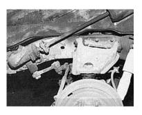
Aside from maybe the heavy accumulation of dirt and grease, this is what your stock, manual steering assembly looks like.
