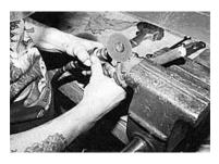
Because of the odd angle in which the rivets are placed, an air cutting wheel is used to cut the head of the rivet off.
