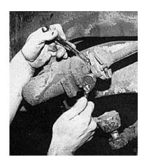
Obviously the first thing to do after you have properly jacked the truck up and secured it with sturdy stands, is to remove the old stock gearbox and pitman arm.
