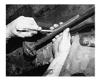
To make sure that you scribe a straight line, C.P.P. has included a one-half-inch section of angle iron that is to be used to make a line as shown. This will keep the correct timing of the shaft after it is cut.
