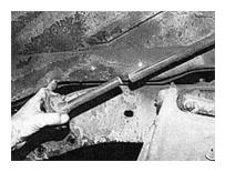
Use a cutting wheel to cut the steering shaft approximately six inches up from the rag joint coupler.
