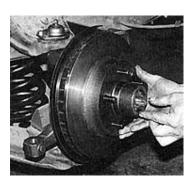
13. Install the new rotor and the outer bearings with plenty of grease.
