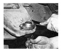
7. After the old ball joint is removed, install the new version. The nuts and bolts are provided in the kit.
