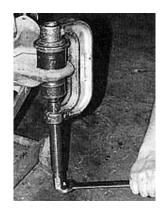
5. Now press the new ball joints which are a '73-'80 version into the lower control arm.
