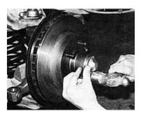
15. A hammer will be needed to install the bearing cover. It is important that you don't forget to put the cover on because any dirt or metal shavings can severely damage the bearings.
