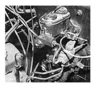
32. The 1967-'70 truck fans will recognize this; it's the manual brake master cylinder from the stock brake system. After this truck was converted to disc brakes, we opted to convert the system over to power.
