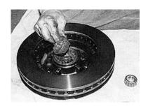
12. Now you can grease-up the wheel bearings and install them into the rotor.
