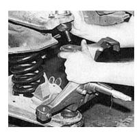
9. You will have to rely on the floor jack once again to press the coil spring together so that the new dropped spindle can be installed. Make sure that the coil spring is set properly into the control arm before you continue.
