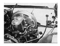
41. This is what the power brake assembly looked like from the factory in 1972. You will notice that there is a support bracket extending from the power booster bracket over to the firewall. Now, the 1971 and '72 firewall designs are different from 1967-'70. The fuse block, parking brake and speedometer cable are located in different places.
