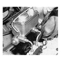
37. The new proportioning valve comes completely assembled with required hardlines, fittings and installation bracket assembled. The mounting bracket simply slides onto the booster stud
