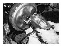
36. Making sure that the pressure pin is still inside the power booster (it likes to fall out if you're not careful), the new power master cylinder can be installed.
