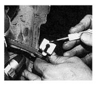
18. The brake fluid hose bracket that attaches to the spindle should be trimmed for a perfect fit.
