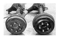
30. If you chose to ditch the stock six-lug rear end to go with a five-lug rear end, a 1971 or '72 half-ton truck will provide you with a good donor rear end.
