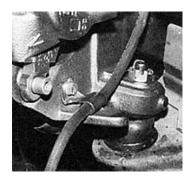
20. When enough excess is trimmed-off, bolt the bracket to the spindle.
