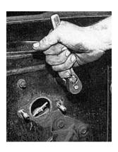
33. The manual master cylinder is attached only to the lower two bulkhead studs. Remove the master cylinder and the nuts attached to the upper bulkhead studs.
