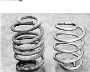
29. To lower the rear suspension to meet the new lowered height of the front, a set of C.P.P lowered coil springs are installed in place of the stockers. You can see the difference which is measureable to a four-inch drop.
