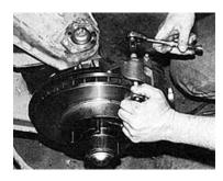
16. Now the calipers can be bolted-up. Installation of the brake calipers requires an allen wrench.
