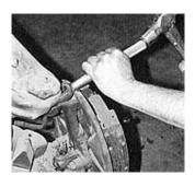
1. To make the installation a little easier, we removed the front sheet metal but you don't have to. To begin, loosen (but do not remove) the stock ball joint nuts holding the spindle on. You will probably have to use a fork bar to get the spindle loose. For safety, release the coil pressure by keeping a jack under the lower control arm, using the truck's weight to hold the spring in place. Warning! you can injured if this isn't done right.
