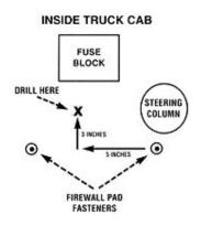
42. This diagram shows you how to drill the bracket hole precisely where you will need to for the 1967-'70 Chevy trucks. Looking from the inside at the firewall, measure over five inches from the pad fastener closest to the steering column, then measure upwards three inches and drill.
