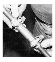
23. Use the new tie-rod end sleeve provided in the kit and install as pictured.
