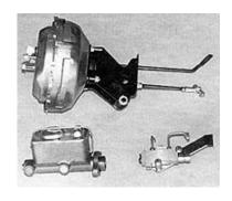
31. It is important that you consider installing a power brake booster, master cylinder and proportioning valve. A '73-80 version bolts-up nicely as does a '71-72 version. The only difference is that the '71-72 version requires a slightly longer thrust rod. This is Classic Performance Products' new power brake kit that comes complete with everything you need to complete the conversion. Trust me, this setup will stop your truck very effectively!
