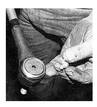
22. Because of the positioning of the old outer tie-rod end when placed on the inside, the kit provides a 90 degree zerk fitting to make lubing access much easier.
