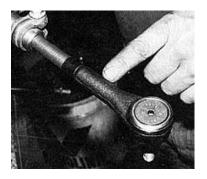
21. Here is where you must pay close attention to the instructions. The kit provides a new outer tierod end and custom made sleeve. The old outer tierod end will now become the inner tierod end if it is still useable.
