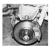
28. There you have it, disc brakes, and a lowered suspension. The suspension is actually lowered about 3 1/2 inches from stock. Now head to an alignment shop to insure proper tire wear and tracking.
