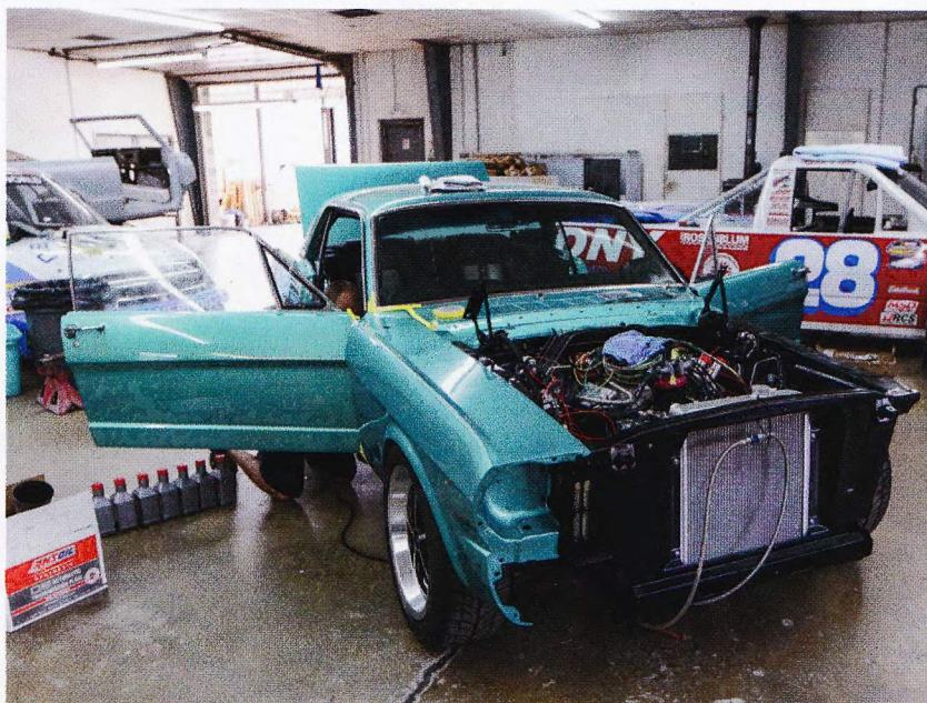
■ This is how we leave Project Road Warrior for this month, in the shop at Mojo Performance. Still left to do is install the Holley Terminator electronic fuel injection system and tune it, tune the Performance Automatic transmission with the MSD controller, wire the entire car ... and about a zillion other small details, as with any complete build.
