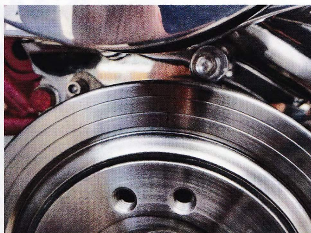
■ The Eddie system could not be used with the large 6.6-inch FPRP damper that came on the engine, since it interfered with a water pump bolt that couldn't be ground for clearance. Since this is an internally balanced engine there were few options in the way of off-the-shelf dampers that would work. Fortunately, Pioneer manufactures an SFI unit of the correct dimensions, and that's what was chosen for this project, courtesy of Summit Racing. After a quick measuring of the press fit, the damper was installed without effort.
