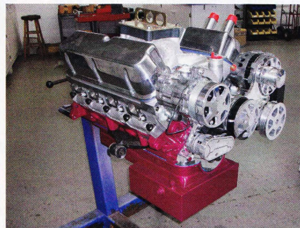
■ We had to use some 0.125-inch shims to get the alternator and power steering pump aligned correctly. The Eddie Motorsports kit looks sharp!
