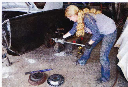
■ CPP also supplied a set of rear disc brakes to replace the stock drums. The Mustang has a Ford 9-inch rearend Barber found (again) in a junkyard.
