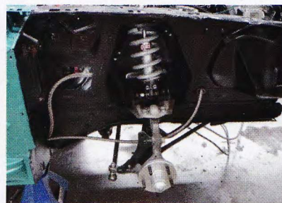
■ Also leftover from the previous build were the Speed Direct bolt-on coilovers and rack-and-pinion steering upgrade. These worked so well that Barber left them alone.
