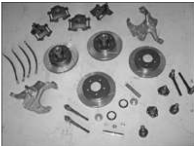
The key to stopping, the Classic Performance Products four-wheel disc deluxe brake kit.
