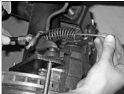
Once the calipers are bolted up, I could then install the new CPP e-brake cables to the calipers.
