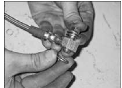
When bolting the stainless hoses to the calipers, be sure to use the provided copper washers for a secure fit.
