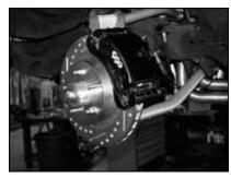
This powerful yet inexpensive front brake upgrade for Chevelles will give us years of worry-free service. These parts are designed to handle weight multiples several times the mass of our Chevelle, which make it safe for any hardcore road course work we
