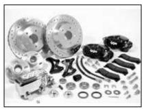
The front brake kit from CPP fits all '64-72 Chevelles (Part No. 6267WBK-P1), and includes 13-inch rotors, dual 52mm piston calipers from PBR, hoses, hardware, mounting brackets, hubs, bearings, seals, cotter pins, pads, and instructions. The chrome master cylinder (part No. CP31500-C) is not included, but if you're upgrading from drum brakes, it's recommended.
