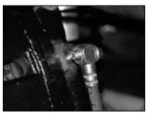
The Chevelle CPP brake kit comes with new rubber brake hoses standard, but Teflon-lined stainless braided lines are available as a \$50 upgrade. Regardless, the banjo bolts (hollow bolts that pass brake fluid) need to be installed with new copper crush washers (included). These washers are dead soft, and are designed to conform to the surface for a perfect seal. We recommend that they not be reused if for any reason you need to take the hoses off.
