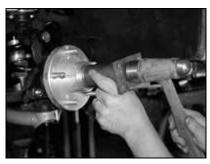
Install the outer seal with a dead-blow hammer and a piece of pipe. This will keep the seal square with the hub. Don't cave in the dome of the outer seal with the hammer.
