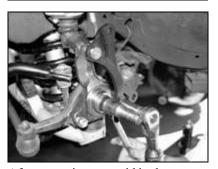
After removing your old brakes, start by installing the CPP caliper mounting bracket. Note that if you are converting from drums to discs, you'll first need to convert to disc brake spindles (Part No. 6474SP-S, pair). Two bolts-a 3/8-inch upper anchor bolt, and a 1/2-inch lower mounting bolt-are a cinch.
