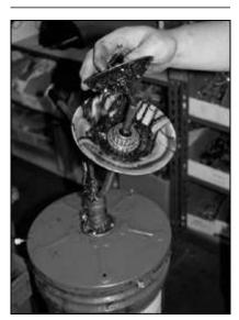
Pack the wheels bearings with highquality high-temp disc brake bearing
