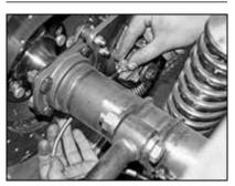
We're going to start from the back of the truck and work up. First, we need to install CPP's rear braided brake lines. If you have drum brakes in the back of your truck, you'd obviously run the hardline to the wheel cylinders.
