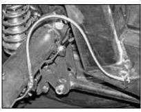
With all the lines on the rearend bent and flared, it was time to pick a spot for the braided flex line to go to the frame. Again, you can weld the tab to
