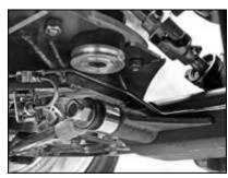
With the tube successfully bent around to the left side of the frame, I ran into a tight spot under the T-fitting's motor mount.
