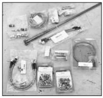
Let's see, we need five brake hoses, a handful of fittings, 30 feet of 3/16-inch hard brake line, and a couple dozen brake clamps to get started plumbing the brakes on the '68. These parts came from both Inline Tube and CPP.
