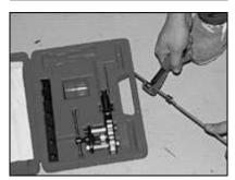
Using my CPP flaring tool kit, I cut the tube on my mark. Do not use a dull cutter, as it can harden the end of the tube.
