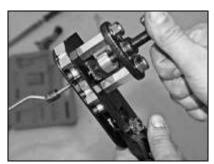
There are two steps for inverted flares: making the first flare that gives the end of the tube a bulb shape, and inverting the first flare. Get it, inverted flare? Both CPP and Inline Tube can set you up with flaring tools.
