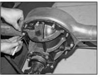
After making the 90-degree bend, I held the bend tightly to the rearend and firmly bent the tube along the edge of the third member by hand. Even though it sounds crude, this is about the easiest and best-looking way to get the job done-just make sure you bend it once.
