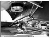
The brake line spanning the front crossmember and joining the front brakes together can be the most intricate and tricky line you'll have to deal with. Because of confining spaces, once a few bends are made it gets difficult to test-fit this piece until it's almost done. Measuring and mapping out the bends helps, and bending up a sample out of a wire
