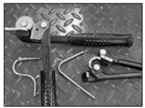
Tubing benders can be a necessary evil to some, but if you get a good one and learn how to use it, it can actually make bending tubing fun! Seriously. On the right is a typical "cheapo" parts store tubing bender that handles multiple sizes and can do the job in most cases, but if you want to get serious and buy a bender that not only works well but should last the rest of your life, get one like this "professional" single-size bender from Inline Tube.
