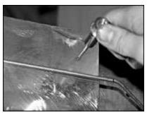
Once you pick a spot, carefully drill a hole with the #21 drill bit, then carefully run a lubed 10-32 tap into the hole. Take your time and don't force the tap, because if it breaks in the hole, removing the hardened tap is not going to be fun.
