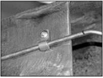
Generally, put one clamp at each end of each piece of tube to hold it in place. When you're done running the rest of the lines, add more evenly spaced clamps.
