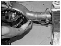
After making the 90-degree bend, I held the bend tightly to the rearend and firmly bent the tube along the edge of the third member by hand. Even though it sounds crude, this is about the easiest and best-looking way to get the job done-just make sure you bend it once.
