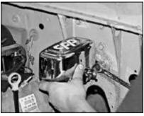
CPP's master bolts right up to the stock location on the F-100 as well as most vehicles. remember, I'm setting up the '68 with manual four-wheel disc brakes, but the master can be used with a booster for trucks with power assist brakes.
