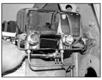
Can't forget to install the brake light switch. From here, if I wasn't going to tear the truck apart for paint, I'd fill and bleed the system. Get on the horn or your computer today with Inline Tube and CPP and round up the parts you need to release your inner plumber!
