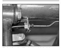
Tada! Looks like it should, huh? Again, to meet up with the brake hose, I made two 45-degree bends in opposite directions prior to reflaring.
