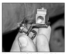
The rearend T-fitting has this little bracket attached to it, and to make it easy to mount, I tacked a 1/4-20 bolt to the rearend that'll be permanently welded once I'm sure it's in the right spot. Now we can bend up the hardline for the rearend since we know where it needs to go.
