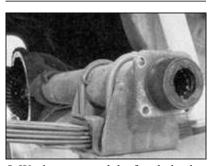
5. We then removed the four bolts that held the old drum assembly to the axle flange and were rewarded with a clean slate to start installing our new parts. We also took a moment to inspect the axle bearings for wear.
