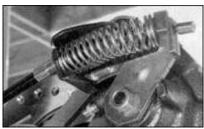
11. With the caliper installed, we connected the new e-brake cable and ran it back to the rest of the system. It was extremely hard to get the Clip on to secure the cable to the caliper, but we got it done after a flurry of curse words. On the otherside, we figured out that it was easier to do with the caliper off the car.
