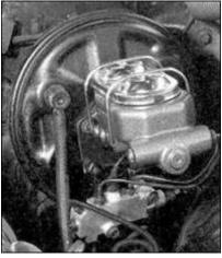
21. After bench bleeding the master, we installed it onto the Camaro along with the new CPP proportioning block. The process was drama free, and when we were done we were able to bleed the whole system and get the Camaro back on the road. The total installation of the rear kit and front parts took all day, with most of that time spent converting the rear drums to disc. Now we just need to get the rest of the second gen looking as good as the new brakes.
