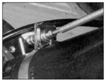
12. In an effort to make this install something you could easily do in your driveway, CPP includes these cool little brackets for the brake lines. By using the supplied band clamps, you don't have to do any welding during the install. Sweet!
