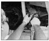
4. With the axles removed, we took the easy route and just severed the old e-brake cable with a cutoff wheel. Since the CPP kit came with new rear e-brake cables, this was the fastest way to get the old junk off. CPP provided new brake hard lines, so we removed the old ones as well.
