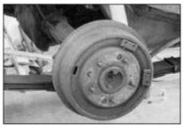
2. While drum brakes do get the job done, they aren't the best looking behind a sweet wheel. They also lag in perfonnance when compared to modem disc brakes, especially after repeated hard stops. The rear disc convernion kit from CPP ran \$599, and we upgraded the caliper finish for \$50 and the rotorn for another \$75. Everything needed for the conversion was in the kit, including brake lines, e-brake cables, hardware, and gaskets for 10- or 12-bolt differential covers.
