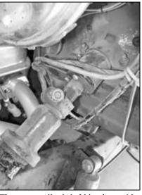
The upper collar is held in place with a single-bolt clamp; once undone, the intermediate shaft can be removed for good.
