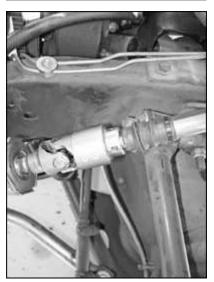
The same goes for the lower application. On the steering box's 13/16-36 output shaft, you'll notice the splines are separated by a recessed groove-make sure the U-joint slips over that, allowing the set screw to lock fully.
