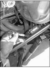
Borgeson provided a 36-inch Double-D intermediate shaft. Oversize, it requires shortening to fit properly. With both U-joints installed, I set the shaft in the lower joint (where it would end up mounting) and marked the spot above where it needed to be cut.
