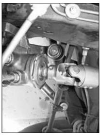
No more rag-joint, that is. The upgrade U-joint from Borgeson is also a vibration damper, so along with absorbing the shuddering, it will compensate for chassis flex as well with the absence of the old slip joint.
