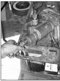
Since the old box was removed with the wheels straight, I took the new Borgeson joint and centered the output shaft before installing the new steering box. In doing so, I realized how much difference there would be when the shaft made one full turn less than the stock one.
