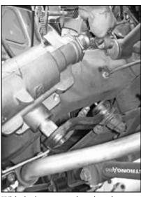
With the box secured against the frame, the pitman arm was ready to be installed. If the splines don't line up just right, reach up and grab the output to manually mesh them with a U-joint.
