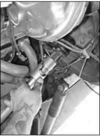
Unlike a setup with varying angles, with the steering box a straight shot below the steering column, you don't have to worry about U-joint bind, so no need to keep the intermediate shaft way below the knuckles. However, that doesn't mean you cram it all the way bottomed out in the joint, either.
