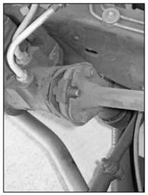
I'm pretty neutral about rag joints. I've never had a problem with one in the past, but still, just the fact that the word "rag" is used in a steering component doesn't sit too well with me. No worries, it will soon join the real rags leftover from the conversion-in the trash.
