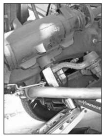
It doesn't matter if you start the removal process at the column or the pitman arm; I chose the latter, making sure the front wheels (suspension loaded) were pointed straight forward before pulling the arm off the box. Typically, the OE sway bar won't cause interference, but if you're using low-profile frame mounts like me, it might get in the way.
