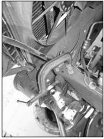
If you're going it alone, secure the box to the frame before removing the last mounting bolt. I did so with a large C-clamp, which worked perfectly.
