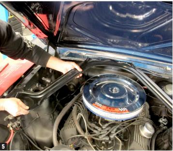
4. Fit the new Export Brace onto the shock tower mounts; capture with the shock tower caps bolted loosely in place. (Figs 5-6)
