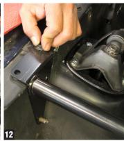
5. The top portion of the brace will bolt directly on top of the firewall/cowl seam (as opposed to beneath, as with the two-piece brace) in the existing four holes. Use a punch to help align holes if necessary. (Figs 7-8)
