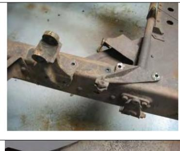
Start by removing the front stock spring hangers and e-brake cable bracket. To remove the rivets holding the brackets, grind the rivet heads flush. Center punch the rivet and drill through using progressively larger drills up to a 5/16" drill. The rivet should be relatively easy to punch out. If it is not, then continue drilling with a 3/8" drill. Take care not to drill the original rivet holes larger or off center, as you will be locating your now parts with these holes.
