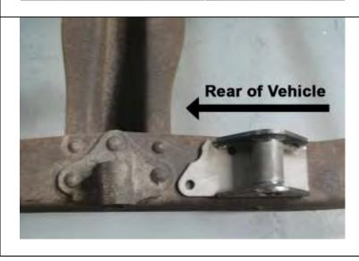
Remove the stock rear shackle bracket rivets in the same manner as the front spring hanger bracket rivets. The shackle brackets are positioned on the rails with the welded side on the inside of the rail. Line up the brackets with the holes of the original brackets. It may be necessary to align-drill a couple of these holes. Use three  $3/8-16 \times 1-1/4$  bolts, nuts, and one washer under each nut to fasten each bracket. The square front edge of the bracket faces to the front of the vehicle.
