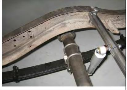
As pictured above, draw a line 28-1/8" in front of the rear bed bolt hole on top of each rail. Center the shock cross member on the top of the rails and mark the hole centers on the lines just drawn. Drill holes through the rail perpendicular to the surface. Drill only the top of the rails and then set the cross member in place and use a transfer punch to mark the hole centers on the bottom of the rail.
