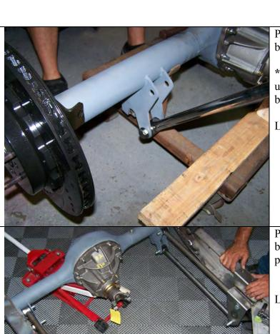
Place the lower 4-link bars onto the lower hole of the axle bracket using the provided 5/8" hardware.
