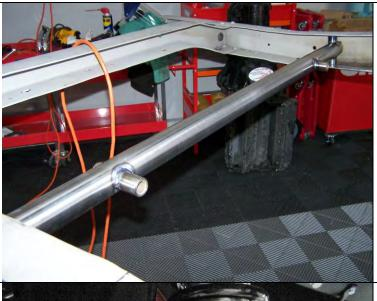
Place the new coil-over cross member into the frame rail with the extended tube for the shock mount pointing forward.
