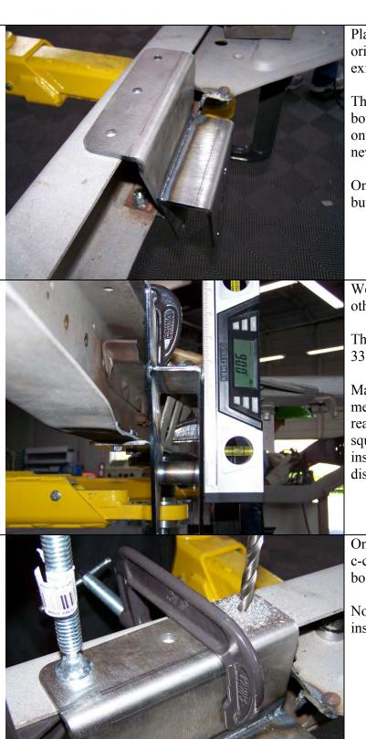
Place the 4-link frame brackets onto the frame where the original front spring perch used to be making sure the existing holes line up.
