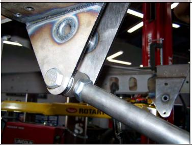
Install the 4-link bars with the adjuster side onto the frame using the provided 5/8" hardware. The bolts are installed from the outside of the frame on the lower holes and from the inside of the frame on the top holes.
