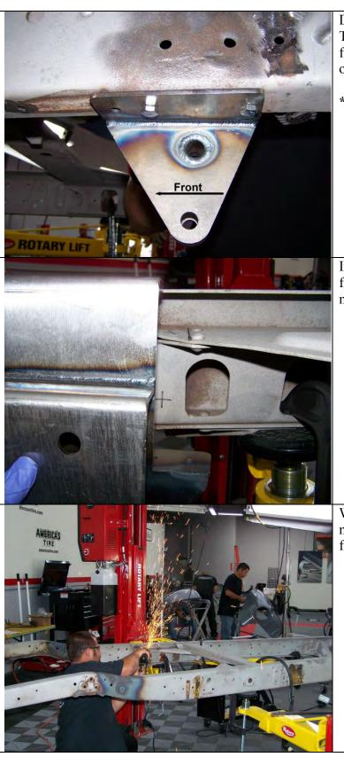
Determining left and right side brackets:
