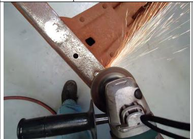
Remove the front leaf spring mounts by grinding off the rivet heads and then punch the rivets body through the frame.
