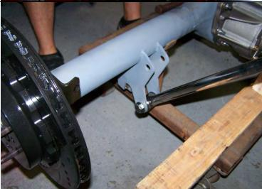
Place the lower 4-link bars onto the lower hole of the axle bracket using the provided 5/8" hardware.
