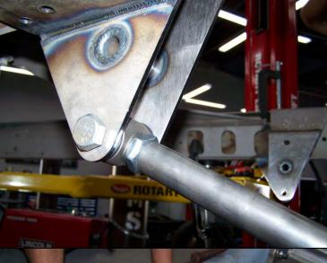
Install the 4-link bars with the adjuster side onto the frame using the provided 5/8" hardware. The bolts are installed from the outside of the frame on the lower holes and from the inside of the frame on the top holes.
