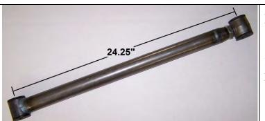
Adjust all the 4-link bars to 24.25" center to center and tighten the jam nuts.
