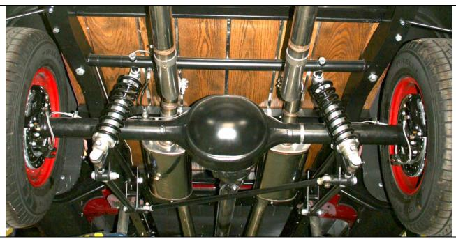
Before removing the stock leaf springs, mark the frame and take measurement as to where the stock axle centerline was. The frame needs to be at the typical 2 degrees rake to mimic actual ride height. Keep the frame at this rake throughout the installation. Remove the brake lines, driveshaft, leaf springs, rearend, rear leaf hangers etc. \*NOTE\* This installation can be done with the bed in place but it will be infinitely more time consuming. We removed it in order to have clearer pictures.
