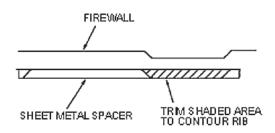
2. If the firewall has a rib, trim the metal spacer to fit as shown in the second diagram. If the firewall is flat, discard the sheet metal spacer.
