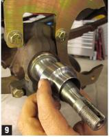
4. Install the supplied bearing adapter onto the spindle; if adapter doesn't fit snug (too loose should require spindle replacement), use green Loc-Tite sleeve retainer. Lightly hit with emory cloth if fit is too tight. (Fig 9)
