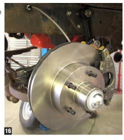
7. Before installing caliper, check slide pin bushings and add grease if necessary. Attach caliper with bleeder screw pointing up. (Fig 13)
