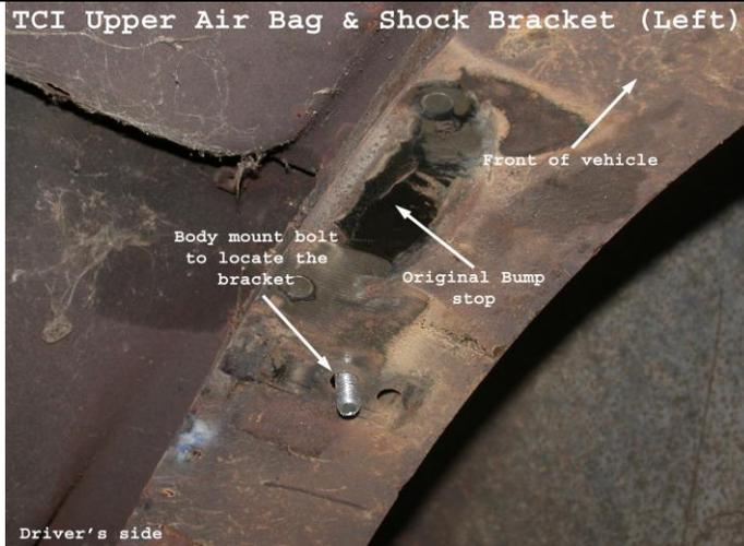
Before installing the rear TCI Upper Airbag Shock Bracket you must first remove the two rivets holding the stock bump stop
