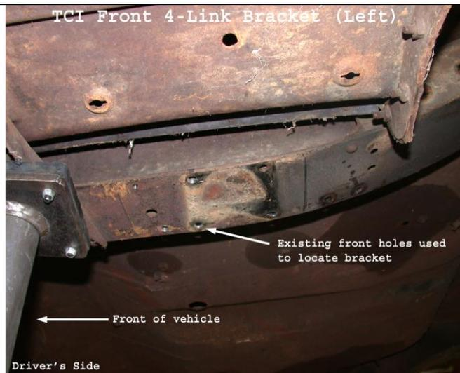
We will start by installing the driver's side front 4-Link Bracket. The four existing holes originally used on the leaf hanger mount will be reused on the 4-link bracket.
