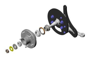
10. Install the bearing dust cap onto the hub. You may need to lightly tap the flange of the dust cap with a small hammer. Avoid hitting the domed part of the dust cap.
