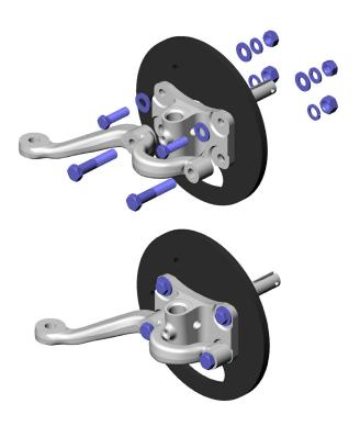
7. Attach the caliper bracket and spacers to the spindle bracket. Two spacers with a flat spot will be used on the upper two threaded holes. The flat spots should face where the caliper will mount. A round spacer will be used on the lower threaded hole. The caliper bracket should hook around the steering arm without interfering. Use three of the shorter ½" bolts (2 ¼") to secure the bracket. A lock washer should be used under each bolt head.
