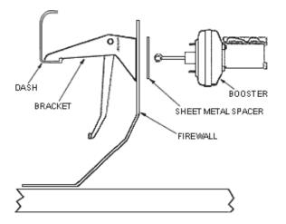
When all the holes are drilled, mount the booster and pedal assembly as shown to the firewall and dash. (Steering column drop mount holes)
