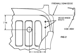
When the brace is removed, a 2-1/2" hole must be drilled with a hole saw 7" from the firewall seam edge and 8-1/2" in from the hood hinge bolts. Mount the brackets to the steering column drop mount holes. Line up the 2-1/2" holes in the bracket and the firewall and clamp in place. Use the bracket as a guide to drill the 1/2" mounting holes.
