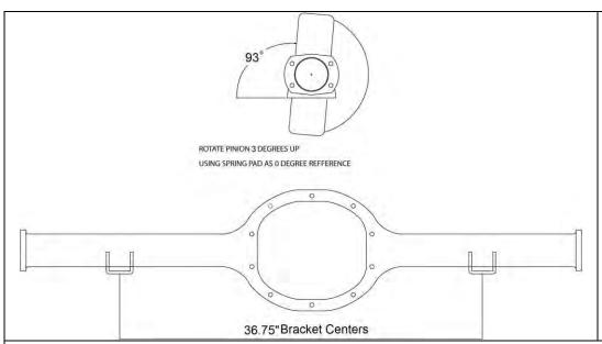
The leaf springs center to center measurement is 36.75". Make sure that both leaf pads are the same distance from the axle flanges on each side so the housing is centered. The pinion angle should be 5 degrees up.
