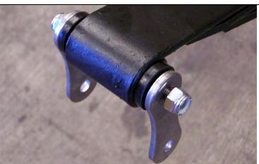
Place the shackle bushings into the rear spring eyes. Slide the shackle pins through the bushings. Place the dogbones onto the shackle pins and install the nylocks.
