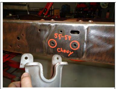
To remove the rivets holding the brackets, grind the rivet heads flush. Center punch the rivet and drill through using progressively larger drills up to a 5/16" drill. Take care not to drill the original rivet holes larger or off center, as you will be locating your new brackets with these holes.
