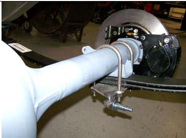
Drop the rearend down onto the top of the leaf springs. Align the hole on the leaf pads onto the stud on the top of the leaf springs.
