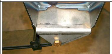
Use the ½-20x4 bolts and nylock nuts to fasten the front of the leaf spring into the front frame brackets. Go ahead and tighten these down.
