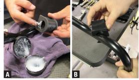
**3.** Position the mounting brackets around the bushings, and with the U-bolts and axle saddle brackets set in place, mount sway bar onto the rear end.
