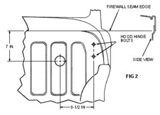
When the brace is removed, a 2-1/2" hole must be drilled with a hole saw 7" from the firewall seam edge and 8-1/2" in from the hood hinge bolts. Mount the brackets to the steering column drop mount holes. Line up the 2-1/2" holes in the bracket and the firewall and clamp in place. Use the bracket as a guide to drill the 1/2" mounting holes.
