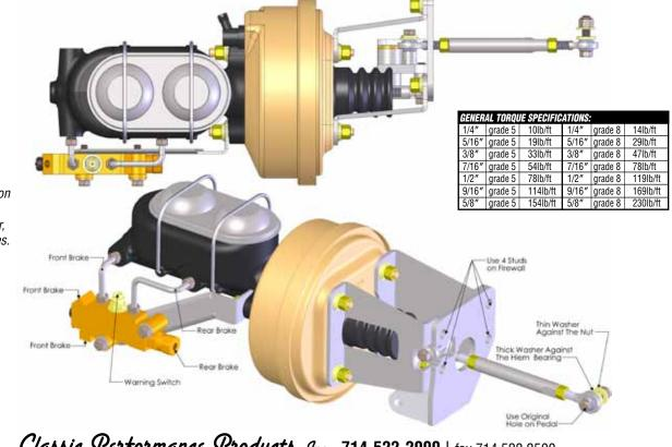
Refer to the illustration in order to correctly assemble the booster, brackets, and linkages.
