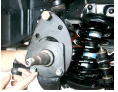
remove the rear steering arm bolt to install the caliper on a later step. Tighten down the top anchor bolt at this time.
