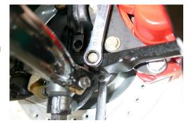
Install the brake hose to the hard line on the frame. Bleed the front brake system with quality brake fluid.
