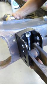
Attach the CPP Anti-Squat brackets using the supplied Grade 8 hardware. (Figs G-H)
