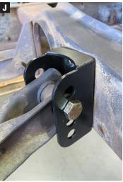
6. Reconnect the trailing arms; use the mounting hole that best corresponds with the amount the rear end has been lowered (the lower the suspension, the higher the mounting hole) to properly set your pinion angle. (Figs I-J)
