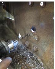
Remove the six rivets attaching each trailing arm bracket. (Figs C,D,E)
