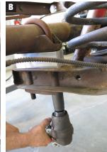
With rear end stabilized, undo trailing arms from the stock crossmember (they may be left installed, but will need to be loose at U-bolts) and rotate the ends downward, out of the brackets. Inspect and replace pivot bushings if necessary. (Figs A-B)
