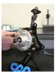
PLEASE NOTE: The installer needs to make sure that nothing can make contact with a brake hose, caliper, or other brake component at any point through the entire range of steering and suspension movement. The installer also needs make sure none of the steering or braking components can become bound or jammed at any time through the range of suspension or steering movement.
