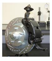
10. Connect the brake hose to the caliper. Use a crush washer on each side of the brake hose fitting. Connect the other end of the brake hose to the brake line and to the frame. Make sure the brake hose has been routed
