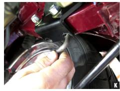
11. Insert lower U-bolts through the bracket and frame. (Fig K)
