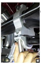
3. Complete axle clamp adjustment, maintaining sway bar alignment; add grease to D-bushing zerk fittings. (Fig M)
