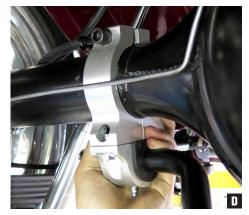
4. For billet clamps, assemble the two-piece axle housing clamp around the axle, with the bolt heads facing toward the rear and the flat D-bushing bracket-mounting surfaces pointing down. The billet lower sway bar clamps cannot be fully tightened until the axle housing clamps are set and tightened, as the Allen heads will interfere with hex bolts. (Fig D)
