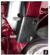
Attach bracket with the end links still connected: install nyloc nuts finger tight. (Fig J)
