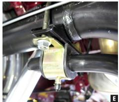
Install standard axle clamp U-bolts onto rear end housing; connect sway bar with D-bushing bracket and lower axle clamp. Dip in bar will be down and towards the rear. (Fig E)
