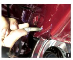
9. Insert the U-bolt through the holes so that the threaded ends stick through the frame on the inside sections first. (Fig I)
