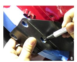
7. Mark the four mounting holes onto the box frame section through the brackets. (Fig G)
