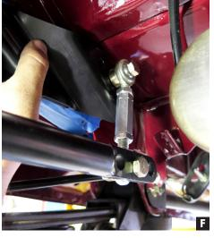
6. Install the Heim-joint end links onto the ends of the sway bar (center hole), and holding bar parallel to the frame and/or ground, determine where the link brackets will attach to the framerails. (Fig F)
