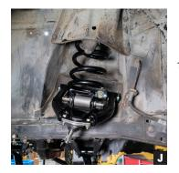
Ensure the spring is properly oriented in reference to the locating tab on the spring perch, then slowly release the tension on the spring. (Photo J)
