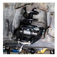
Fasten the shock to the spring perch using the supplied hardware. (Photo L)
