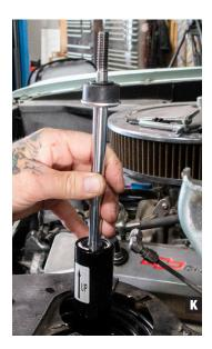
Install the new shock into the shock tower. (Photo K) 15. Repeat steps 7 through 14 on the other side, then have the vehicle professionally aligned.
