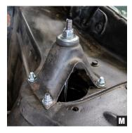
14. Put one of the supplied washers on the top of the shock followed by a bushing. Then re-install the shock tower, add another bushing and washer to the top of the shock, and finally secure with a nut. (Photo M)
