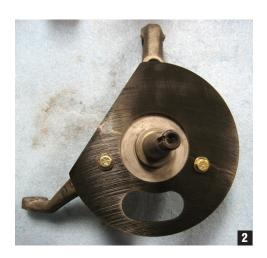
2. Install the backing plate using the two lower mounting holes on the spindle with the supplied hardware. Note: Brackets will fit either side. (Fig. 2)
