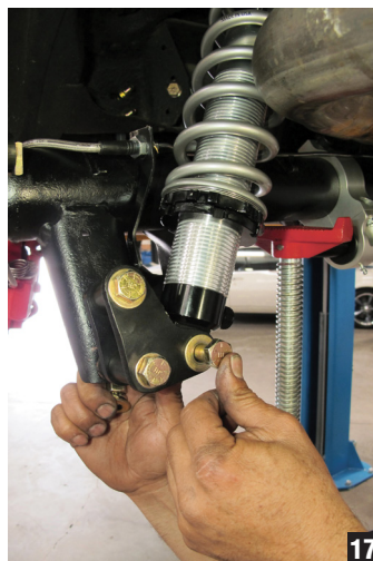
13. With the rear end compressed, attach the coil-overs, making sure the adjuster knob(s) face inward, away from the bracket, so as to allow for future on-vehicle tuning. (Fig. 17)
