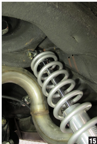
11. With the rear end still safely/securely supported, loosely hang the new coil-overs in the stock upper shock-mounting location. (Fig. 15)
