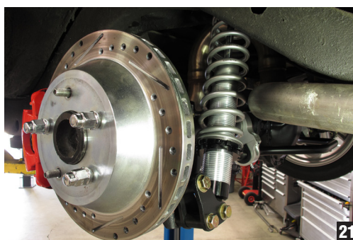
17. Your particular ride height may dictate brake caliper placement in certain applications. Here, with a 12-inch brake kit, the calipers need to be mounted in the forward position to clear both the framerail as well as the coil-over and lower mounting bracket. (Fig. 21)
