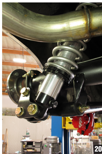
16. The single-adjustable shocks offer 18 individual damping settings—duals have 18 additional adjustment options for rebound as well as compression. Start soft to midway firm (2-8 clicks) and fine-tune your ride characteristics from there. (Fig. 20)
