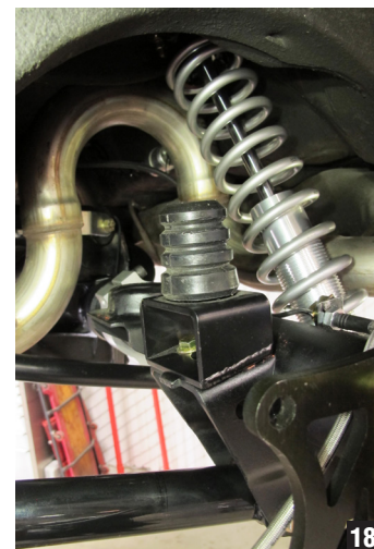
14. Next, mount the new bump stop and accompanying perch onto the rear end in the stock bump stop location. (Fig. 18)
