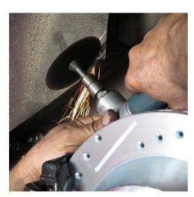
For 1968-69 Camaro / Firebird and 1968-74 Nova / X-body cars, it may be necessary to clearance the drivers side frame as shown to avoid the caliper making contact.
