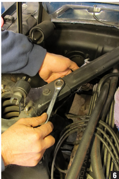
3. Remove the remaining stock braces. (Fig 6-7)
