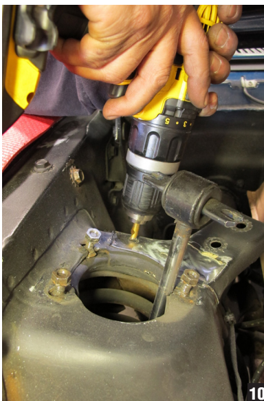
5. This may be done by drilling the spot welds out and carefully cutting the brackets from the towers. Take care not to damage underlying sheetmetal at all costs. (Figs 9-11)
