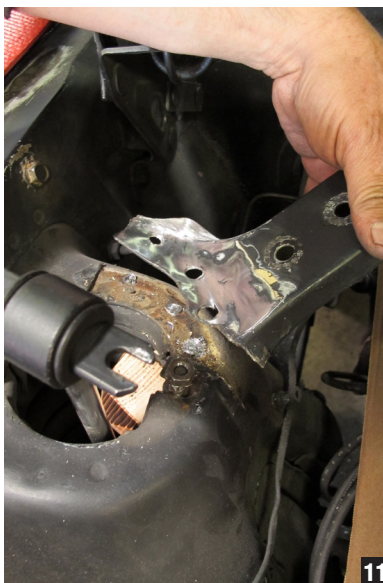
5. This may be done by drilling the spot welds out and carefully cutting the brackets from the towers. Take care not to damage underlying sheetmetal at all costs. (Figs 9-11)
