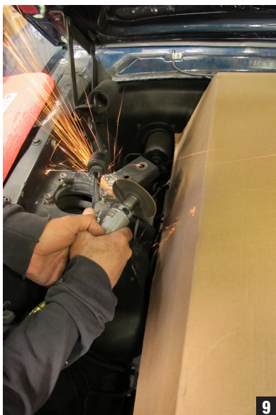
5. This may be done by drilling the spot welds out and carefully cutting the brackets from the towers. Take care not to damage underlying sheetmetal at all costs. (Figs 9-11)
