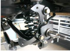
2. With the hardware supplied, install the small bracket to the front side of the spindle using the factory steering arm bolt holes. Install the steering arm at the same time. Tighten down the bracket to the spindle.
