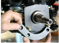
Start by removing either the factory drum brake assembly or your current disc brake conversion from
