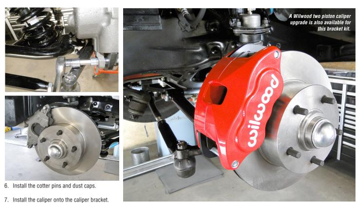
8. Bleed the front brake system with quality brake fluid.
