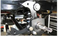
Tighten down the top anchor bolt and bracket bolt now.
