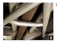
5. There should be sufficient driveshaft clearance, even when rear end is at full sag; however, a worn out transmission mount can/will cause the driveshaft to hang lower, so in the event it rubs, check condition of mount, and replace if necessary. (Fig E)
