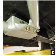
3. The forward tabs go on top of the Subframe flange. (Fig C)
