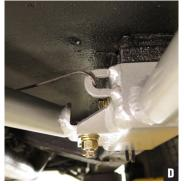
4. Your stock parking brake return spring will clear the top of the X-Brace tube. (Fig D)
