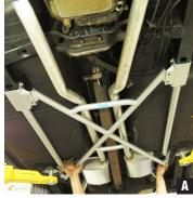
1. With vehicle safely and securely supported allowing sufficient room to work beneath, set X-Brace onto the forward-side Subframe Connector mounting tabs. (Fig A)
