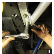
2. The rear tabs will attach from beneath the Subframe flange. (Fig B)
