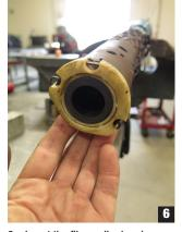
Insert the fiber collar bearing replacement into the plastic retainer-the outside edge must be flush in order for the steering shaft to fit properly.
