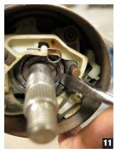
With lower shaft flush against lower fiber collar, install the spring washer, flat washer, and upper C-clip, in the exact orientation as on the stock inner steering shaft. Check for excess
