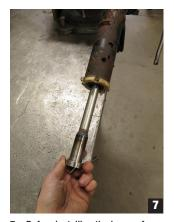
7. Before installing the lower of the two C-clips, test fit the CPP steering shaft to ensure it fully engages into the top, enough to allow the upper C-clip and washers to be installed.
