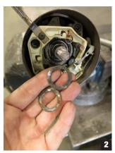
1-2. With stock column out of the vehicle, remove the steering wheel with a suitable puller. At the top of the shaft, just beneath the turn signal assembly (approximately 1-1/2" below the splines), there will be a C-clip retaining a flat washer atop a spring-steel washer. Remove all three.
