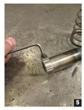
Before installing the new inner shaft, thread the Allen set screw into the steering box input coupler (bottom), just enough so it will not interfere with bearing retainer, but not deep enough to prevent shaft splines from fully engaging with input splines.
