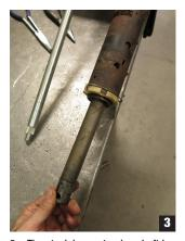
The stock inner steering shaft is now free at the top end of the column and can be pushed down and out through the bottom of the tube.
