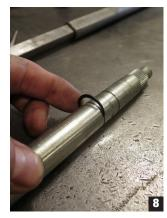
Remove the shaft and install the provided C-clip onto the lower of the two grooves on the upper side; reinstall shaft in column.
