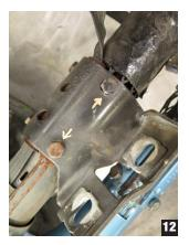
If the upper column bracket will not adjust enough, oblong the holes attaching it to the column until it does
