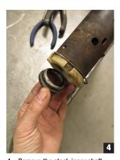
Remove the stock inner shaft as well as the lower sealed bearing; thoroughly clean the plastic bearing retainer, as it will be reused.
