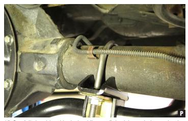
15. Carefully hand-bend brake hard lines to fit back beneath the stock axle tabs. (Fig P)
