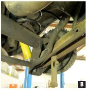
2. If vehicle is equipped with factory (or aftermarket) rear sway bar, remove entirely. None of the stock mounting points and/or hardware will be reused. (Figs A-B)
