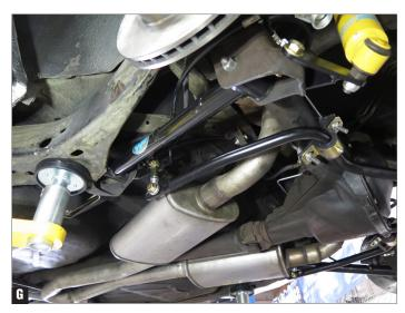
8. CPP's Pro Touring Sway Bar (#7887PTSBK) will not mount off the new trailing arms, as it uses a separate mounting bracket for the adjustable end links. (Fig. G)
