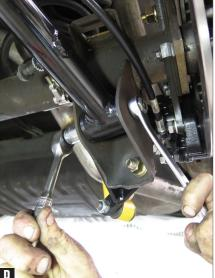
4. Reusing the original hardware, install the new CPP Totally Tubular arm: the threaded bungs (on the rear pivot end of the arm) will point toward the driveshaft. (Fig. B, C, D)
