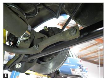
6. To reinstall stock sway bar, attach using supplied M10-1.5x35mm flanged head bolts and serrated lock washers. (Fig. E)
