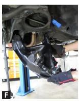
Remove stock upper and lower control arms. Note the number of alignment shims used (though amount re-used will depend on the desired camber) and retain Metric nuts for upper cross shafts. (Fig. E-F)
