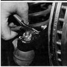
About the only thing left on the steering end of things is to reconnect the tie rod ends. Once everything is where you want it, don't forget to torque all the fasteners to proper specifications and slip the cotter pins back in place.
