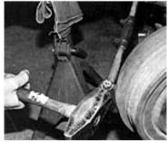
With the car securely supported on jack stands, the first order of business is to disconnect the tie rod end from the steering arm. If you don't want to ruin your tie rod end boot, a few smacks to the side of the steering arm with a heavy hammer should break things loose.
