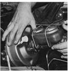
After your brake line situation has been figured out, it's time to install the master cylinder and power booster. while those items come already assembled, we found that, for clearance reasons, it's often easier to remove the master cylinder and install the booster first.
