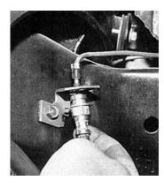
Then the brake line can simply be connected again.
