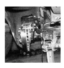
the old braking components. We started by removing the brake shoes and then the rubber brake lines going to the wheel cylinders. Chris had ordered custom emergency brake cables (since the drum brake cables will not interchange), so we disconnected the old cables from their original starting point.
