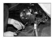
For a clean installation, Chris installed the optional hard brake line kit. With all
