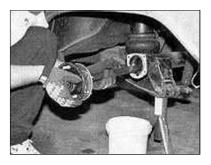
If was determined that our wheel studs weren't long enough for our new brake/wheel combination. We went to the local auto parts store, found the length we needed, and pressed them in. Taking the longer bolts (to accommodate the new caliper bracket), we pre-installed them through the bearing retainer plate and slipped on the metal spacer ring.
