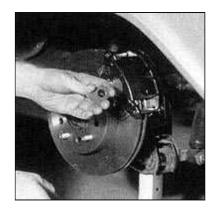
With the major work out of the way (and the calipers on the correct sides), it was time for the final details. The CPP kit includes mounting tabs for the rubber brake lines. For our installation we welded the tabs in place, but you can choose to bolt them in.
