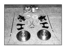
Classic Performance Products offers a complete bolt-on rear disc brake kit for most early Chevys as well as many musclecars. Shown here is the complete rear disc brake kit for '55-64 fullsize Chevys using an original rear axle (power brake booster and emergency brake cables are optional, but also available from CPP). This is a complete kit, with all necessary hardware and instructions.
