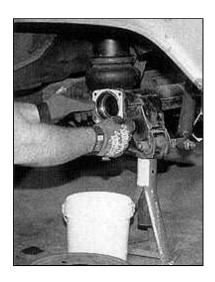
To remove the brake backing plates, you simply undo the four bolts that retain it on the axle. By pulling towards you, it will break loose.
