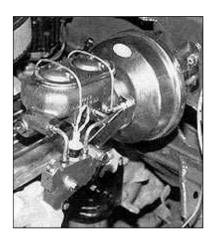
the pre-bending done for us, the installation was very straightforward, resulting in a perfect fit. Having all new brake hardware made installing the new rubber brake lines a snap. To be sure that the emergency brake cables were long enough (or short enough), they were test fit on the car. We determined that the cables were the lengths necessary to operate properly, so we installed them, starting at the caliper side and working our way towards the front.
