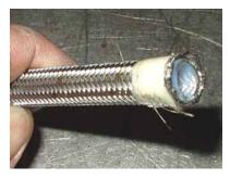
**Step Three:** Slide the female hosenut down onto the hose with the threaded opening oriented towards the cut hose end. Carefully remove the tape from the stainless overbraid. Now take a blunt tipped screwdriver or alternate tool and spread the stainless overbraid away from the inner teflon hose liner about a 1/4".
