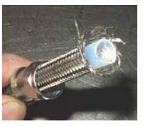
**Step Six:** Grab a suitable tapered punch and expand the teflon liner into the I.D. of
