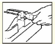
**Step 3.** Lubricate nipple and socket threads. Use a molydisulfide base lubricant for stainless steel fittings (e.g. Molykote Type G); lubricants containing chloride are not recommended. Other material combinations use standard petroleum lubricants. Hold the nipple with hex in the vise. Push hose over nipple with twisting motion until seated against nipple charmfer. Push socket forward and start threading of socket to nipple.
