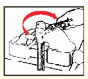
Step 4. Wrench tighten hex until clearance with socket hex is at J031 inches. Your thumb nail is a convenient measuring device. Tighten further to align corners of nipple and socket hexes. CLEAN, PROOFTEST TOTWICE OPERATING PRESSURE AND INSPECT ALL ASSEMBLIES.
