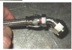
this point. You may now back the hose end out of the hose up to one full turn to orient it in the direction desired. Doesn't this have to be tight? NO! The initial torque down crushes the brass ferrule down a few thousandths, which seals the teflon liner very well against the male nipple of the hose end, which means that you will still seal the joint positively even if unscrewed up to three full turns (!). These lines seal so well that they can also be used with Nitrous without fear of leakage!
