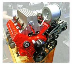
by-wire throttle body which is controlled by a Holley **EFI** system. The billet aluminum fuel rails appear to be periodcorrect with their antique looking brass
