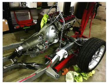
the car in roughly one year using only parts that could be bought straight out of the company's catalog. The foundation for the build began by replacing the worn, stock chassis with a new Art Morrison GT55 chassis. Morrison chassis were relatively new to the market when this car was built originally. The chassis has stood the test of time and has been altered only slightly since they were first introduced. This is a real testament to the design and the company that makes them.
