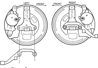
Diagram D: 1962-67 Nova steering arm installation. 1962-63 4-lug Novas must use steering arms from 1964-67 5-lug Novas. (#6267SA)
